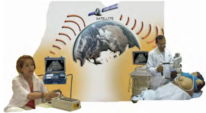
Figure 1: WORTEX intercontinental deployment setting: the health professional controls, via satellite, with a haptic probe the remote MELODY robot positioned by a paramedical assistant on a patient.
